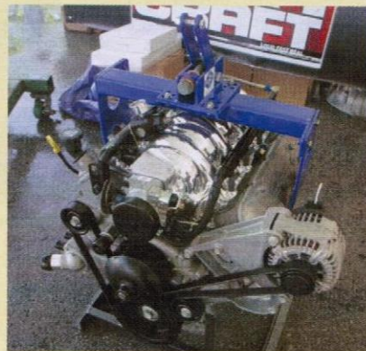
Each team would bolt in one of these GM Performance Parts LS6 engines that Holley had previously equipped and tested with a Holley intake and the new Holley HP electronic fuel-injection system. To assist the swap, Holley fitted each engine with a Mac’s Pivot Plate (PivotPlate.com).
