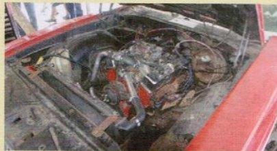
Team Olds’ engine compartment revealed its preparation. The rules required the car to run, but only for a short period, so Justin Dermody bypassed the radiator and had an EFI pump and tank in the trunk. The carbureted small-block was fed by a plastic gas can under the hood, and the battery had been moved to the trunk.
